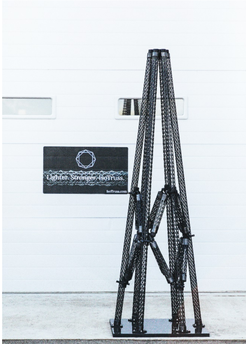
Figure 9. Photograph of the demonstration piece showing the potential for IsoTruss in large wind turbine towers.
