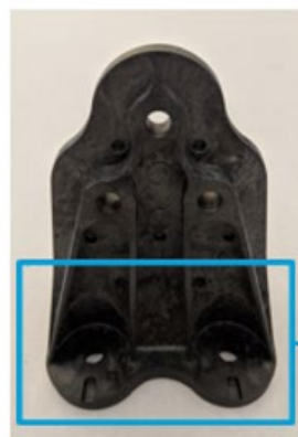
Figure 51 - Doubled Lower Section Preform Design
