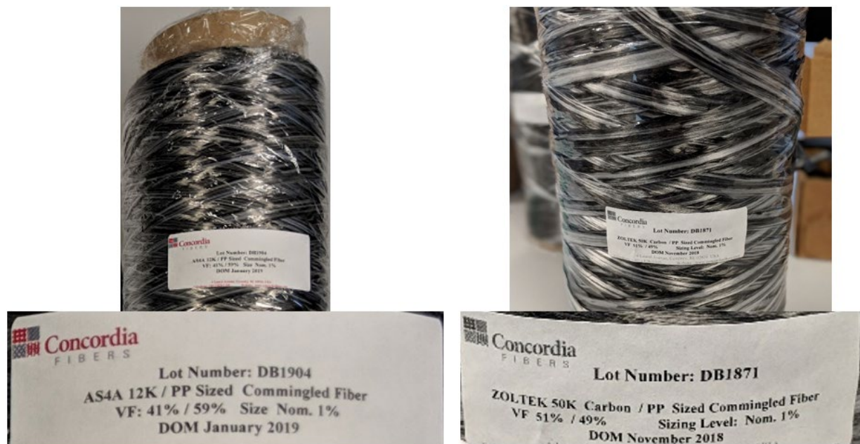
Figure 17 - AS4A 12 Carbon Fiber Commingled with Polypropylene Fiber (Left), Zoltek 50k Carbon Fiber Commingled with Polypropylene Fiber (Right)
