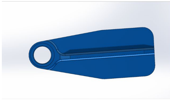
Figure 53. Alternate Airbus bracket used for cost study, approximately 5" x 2"
