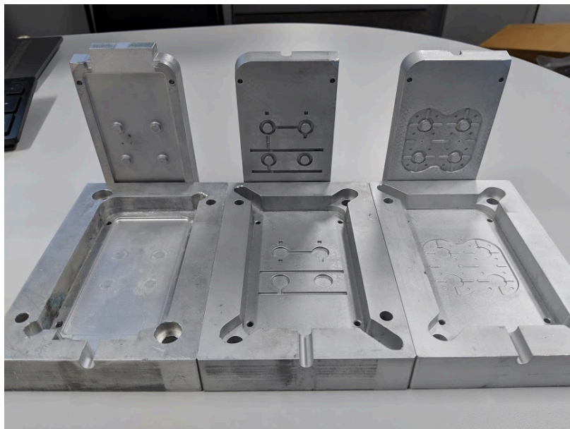
Figure 11 - Flat Plate Tool, 1st Shot Tool Version 1, 1st Shot Tool Version 2 (Left to Right)
