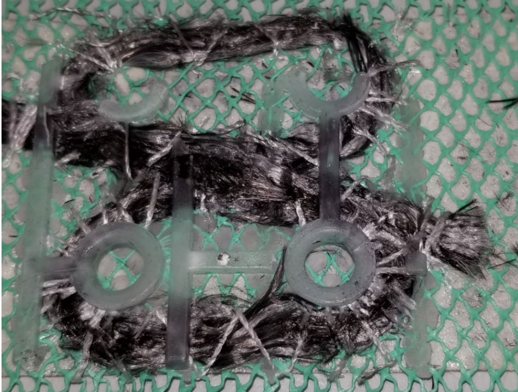
Figure 10 - Injection Overmolded First Shot with Broken Fibers
