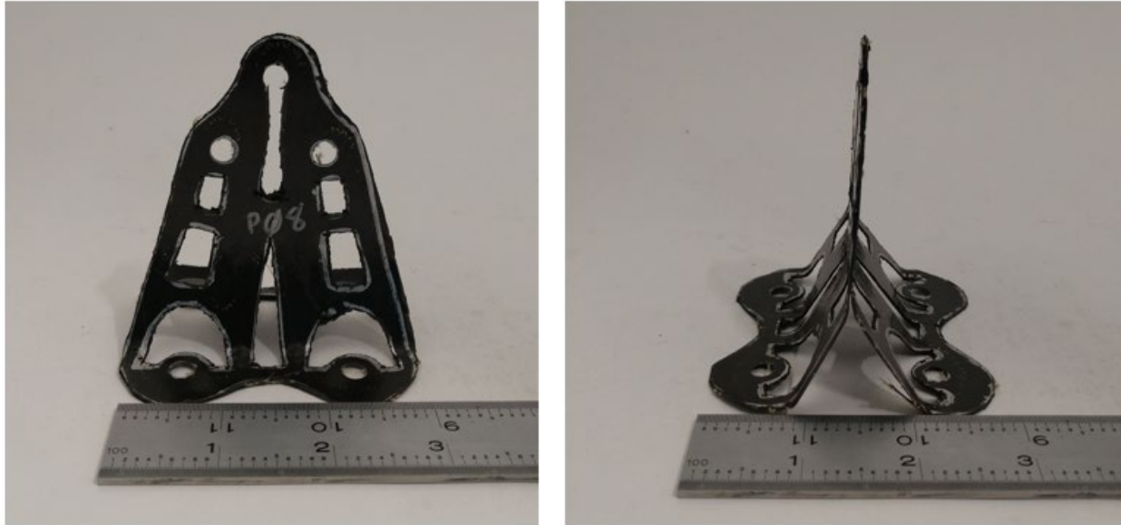
Figure 43 - Hand Cut and Formed Pre-consolidated TFP Preform, Front and Side View
