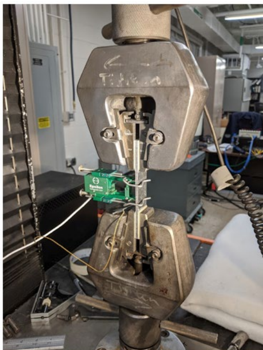
Figure 30 – Load Frame Test Setup for Tensile Tests of Flat Plate Specimen
