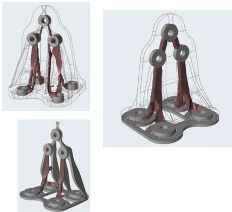
Figure 38 – Topology Analysis Results Used to Determine Fiber Placement for TFP
