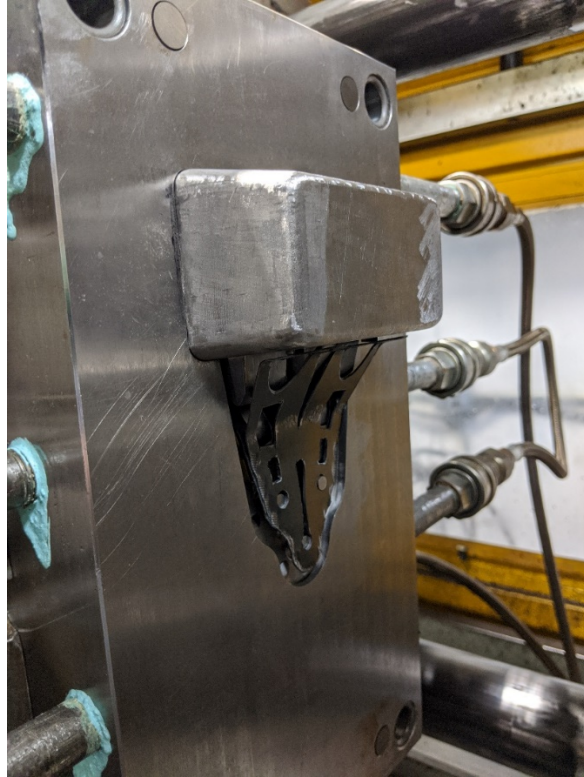
Figure 47 - Preform Loaded into Injection Molding Tool
