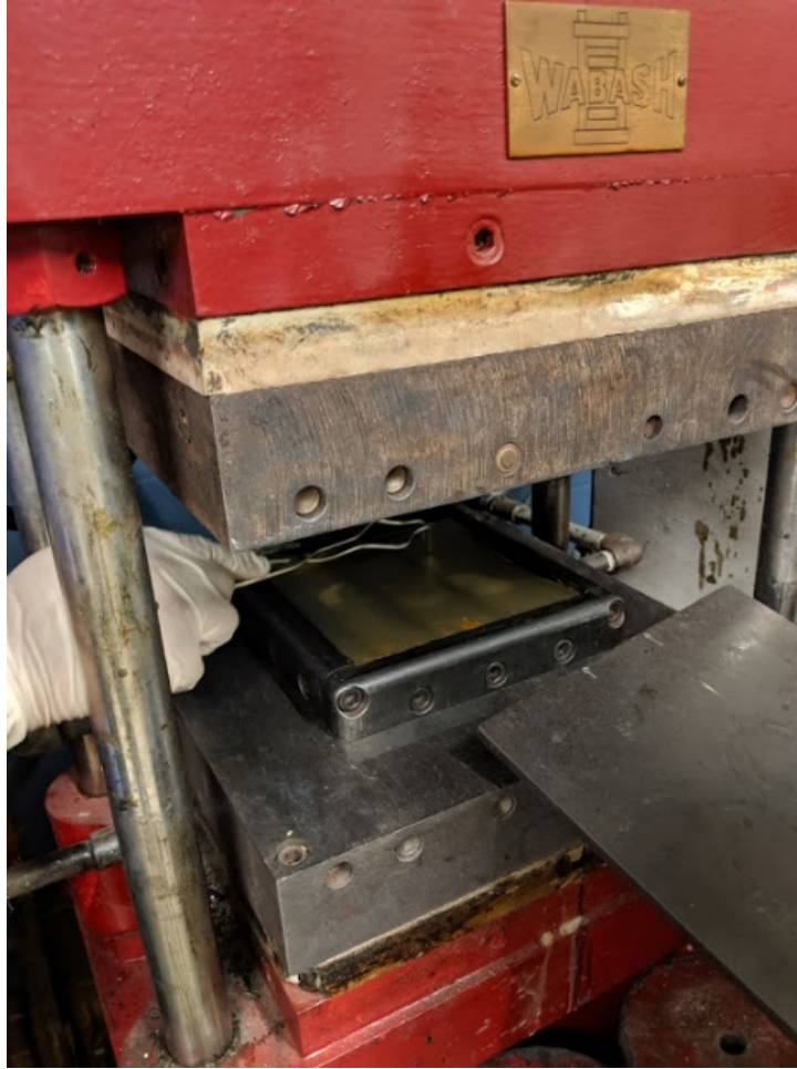
Figure 24 – Film and TFP Layers Pressed Into Pre-consolidated Preforms
