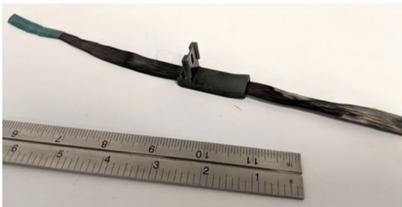
Figure 14 – Limited by the Current Machine a 3D Printed Foot was designed to spread tow
