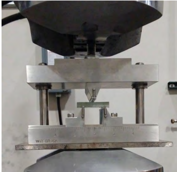
Figure 46. ILSS short-beam shear specimen loaded in fixture.
