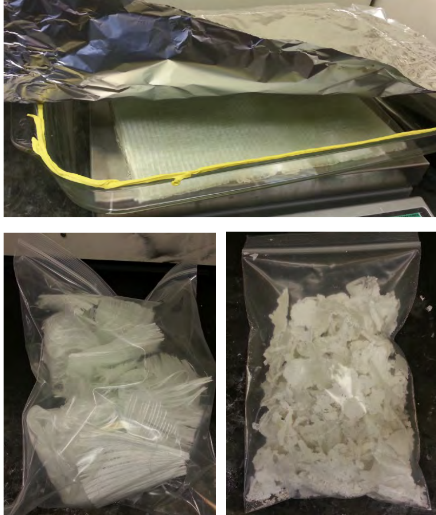
Figure 5. Thermoplastic Elium® composite (top) can be separated into fibers (left) and the polymer resin (right) by dissolution. This separation and recovery is not possible with thermoset composites.
