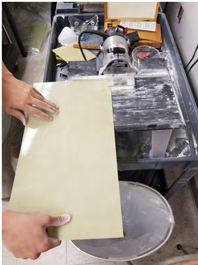
Figure 19. G10 fiberglass material cut into tabs for tensile specimens and select compression specimens using a Tensilsaw model 60-62 with a diamond-plated blade.
