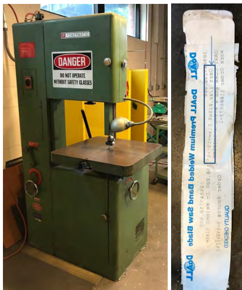
Figure 16. Band saw used to square panels and facilitate XCT scanning to determine fiber orientation.
