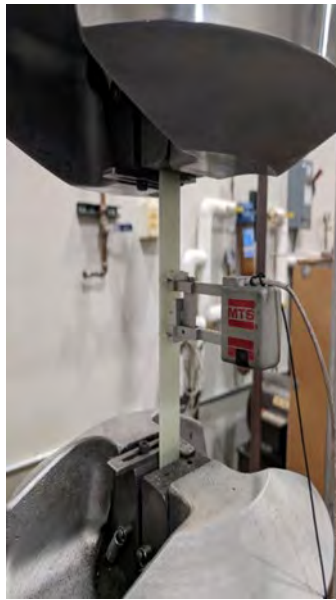
Figure 29. Example tensile specimen loaded in MTS testing machine with extensometer attached.
