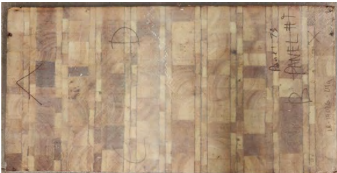
Figure 23. Example of 122 x 61 cm epoxy-gf-facing sandwich panel with balsa core received from TPI.
