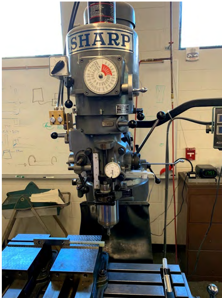
Figure 18. SHARP vertical knee mill utilized for precision cutting of all laminate samples.
