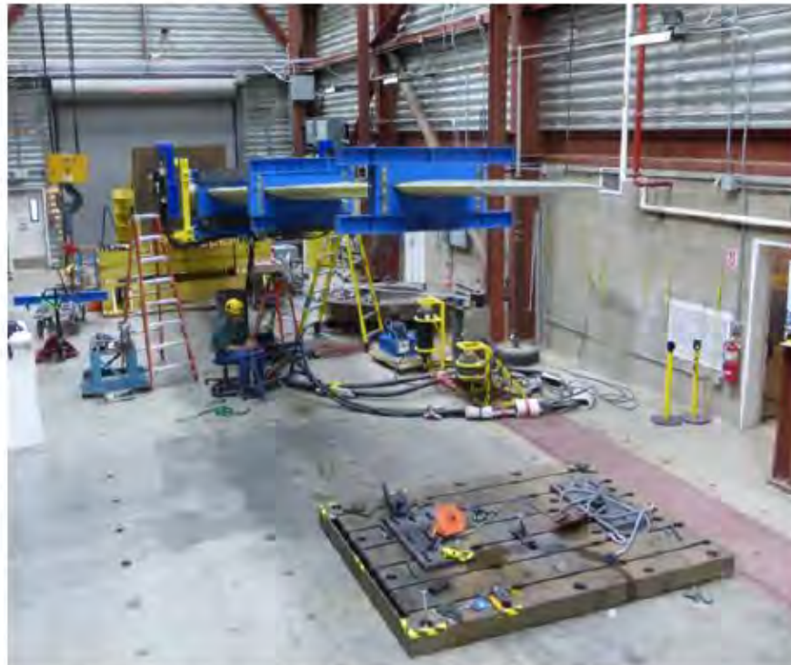
Figure 1. Blade test article and test setup (epoxy blade shown)
