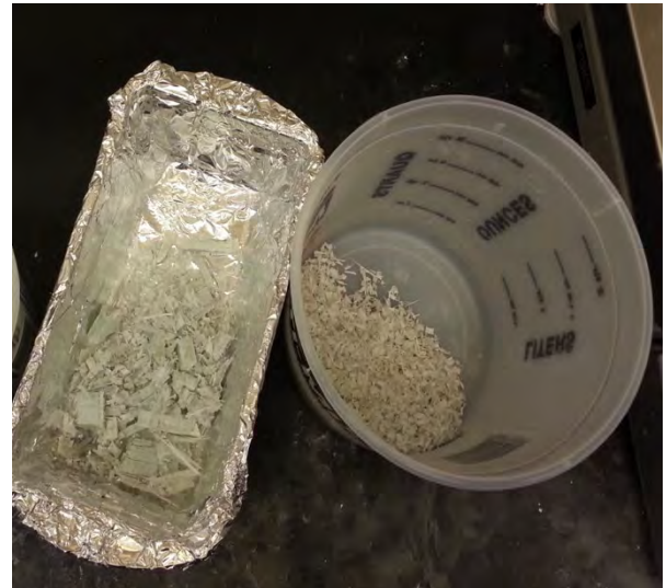
Figure 3. Strips of spar cap component (left) and subsequent ground composite material passed through a 3.5 standard mesh screen (foil pan) and a 7 standard mesh screen (round bucket).
