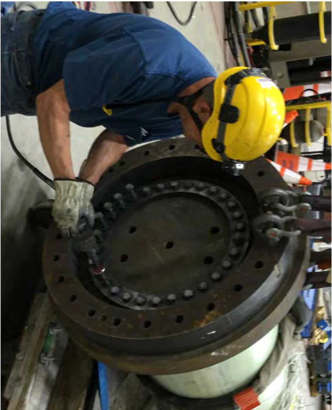
Figure H-1. Adapter Plate Mounting Configuration for Static Proof Load Tests
