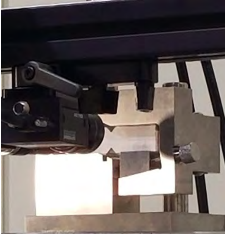
Figure 37. Example of the Iosipescu specimen in the test fixture with a speckle pattern for DIC strain analysis.
