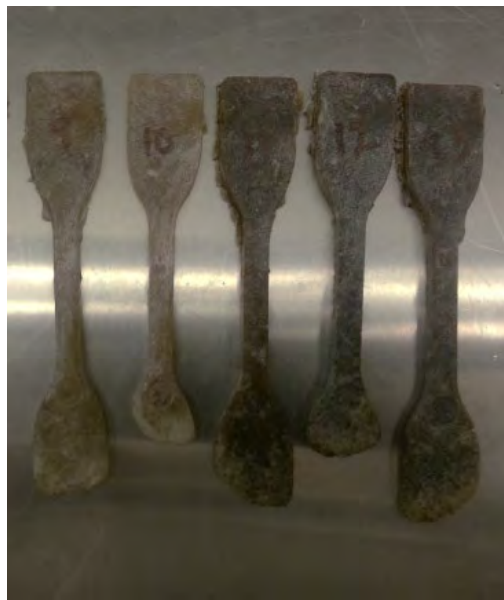
Figure 4. Dog bones fabricated for tensile testing of the regrind material.
