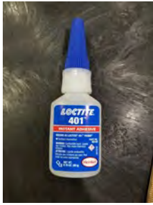
Figure 20. Cyanoacrylate adhesive (Loctite 401) used for bonding tabs to laminate specimens.
