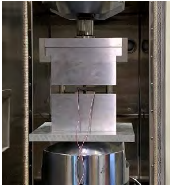
Figure 36. Compression specimen in the IITRI fixture with strain gages mounted to opposing faces.
