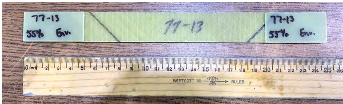
Figure 66. Example GF/Elium® coupon after conditioning at 70°C and 90% RH, before fatigue testing.
