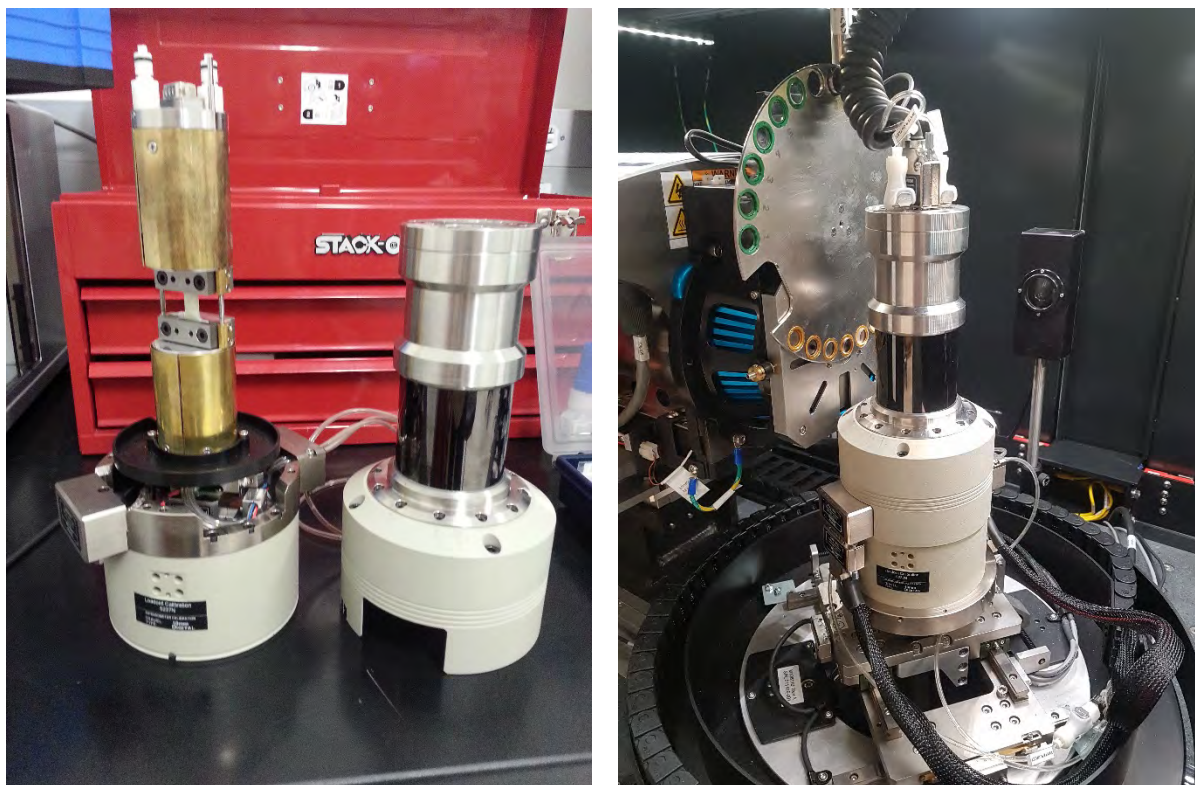
Figure 84. Deben in-situ X-ray computed tomography load frame. At left, the specimen can be seen loaded into the frame and on the right, the instrument is loaded in the XCT cabinet.
