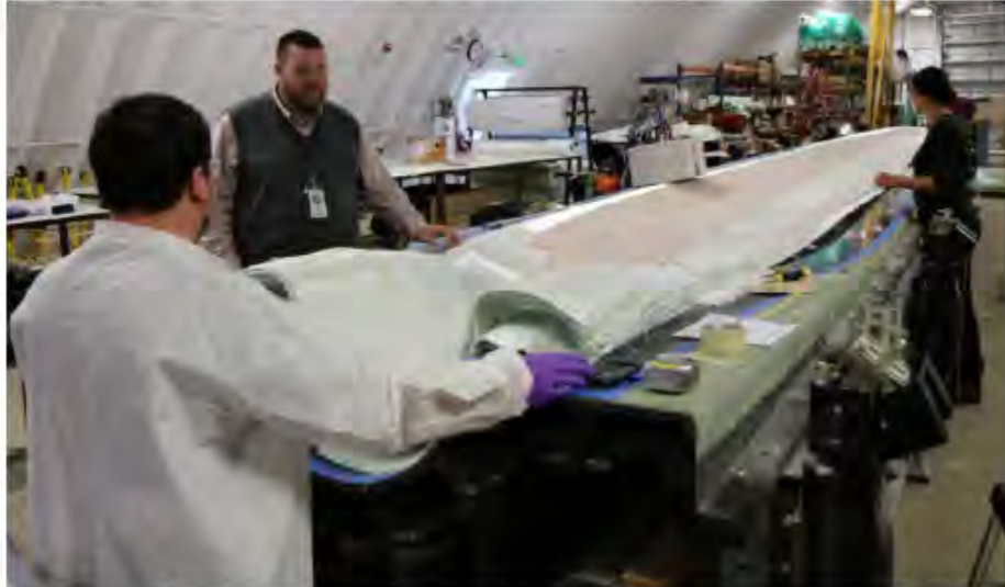
Figure 2. Dry material placement in the mold
