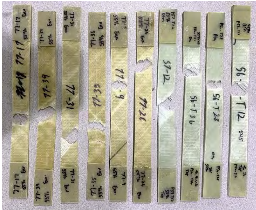
Figure 75. Typical failures for 55% UTS [\pm 45]_s GF/Elium® samples. Discolored samples were conditioned, while white samples were virgin material.
