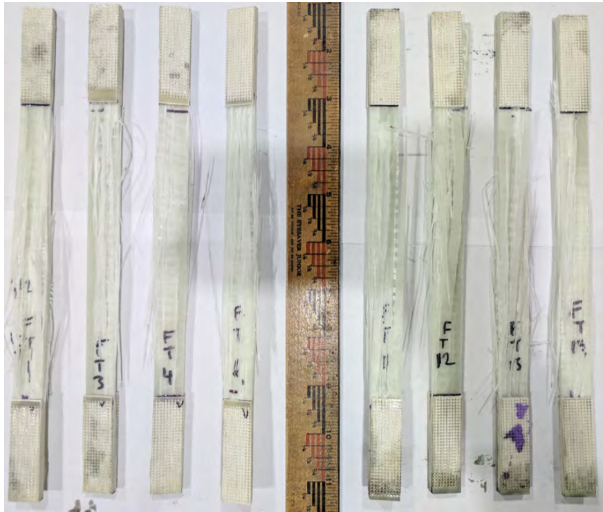
Figure 30. Elum-gf 0 2s samples failed in the interlaminar and interfacial shear coupled with transverse fiber breakage.
