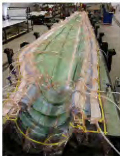
Figure 3. SS under vacuum bag during infusion
