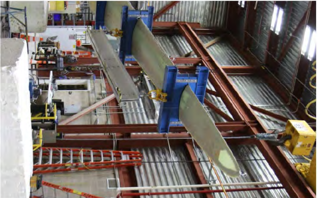
Figure H-3. Max Flap setup showing rigging line from spreader bar to overhead crane
