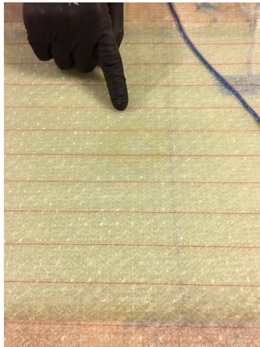
Figure 132. Picture of a cured composite that had a pinhole in the bag that was sealed up during the infusion
