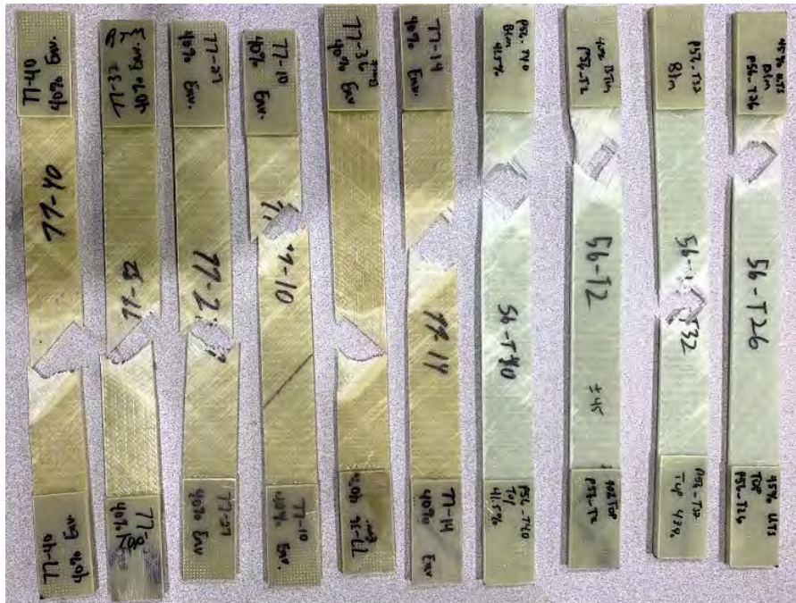
Figure 76. Typical failures for 40% UTS [\pm 45]_s GF/Elium® samples. Discolored samples were conditioned, while white samples were virgin material.
