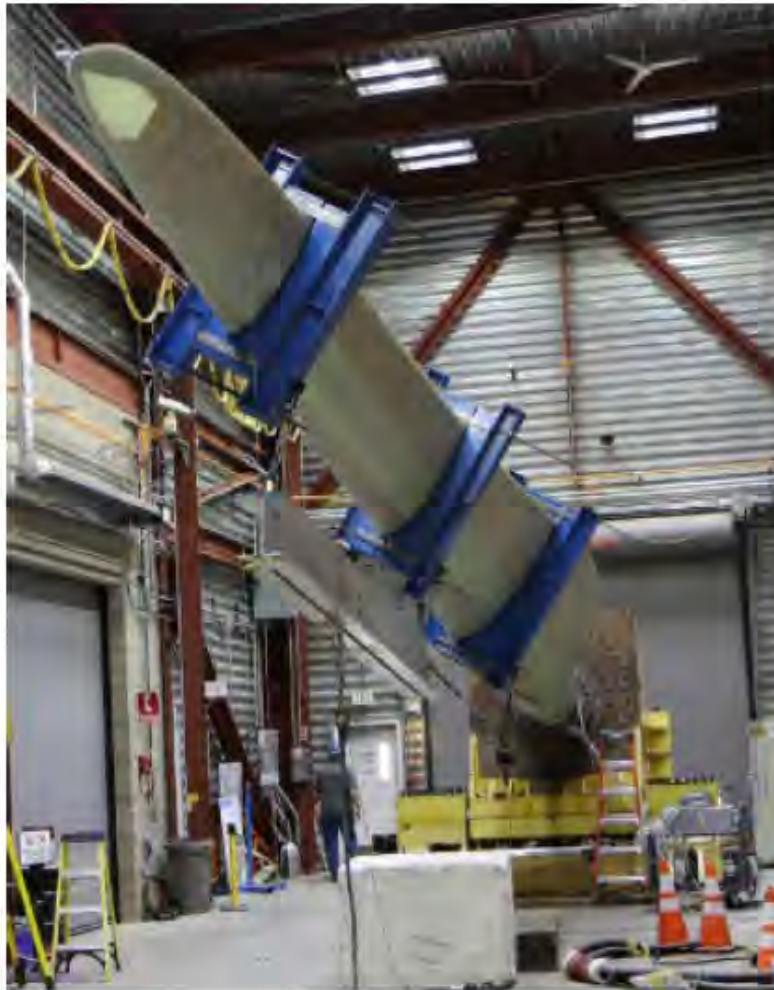
Figure 1.– Maximum Edgewise Static Test Setup
