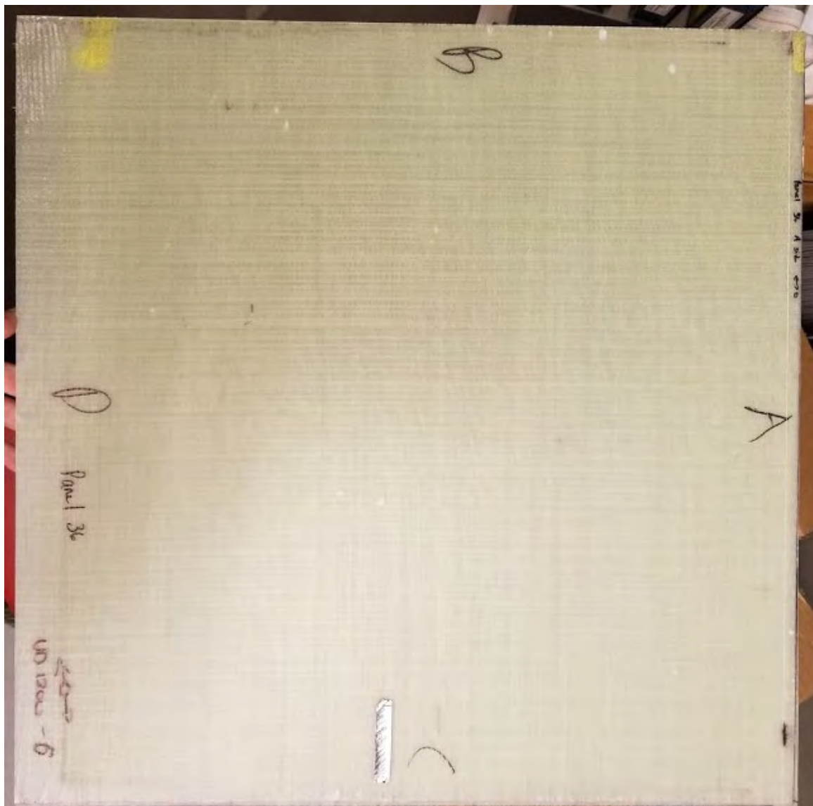
Figure 14. Elium-glass fiber composite panel as received from TPI with lead (Pb) tape applied to mark the apparent fiber orientation confirmed by radiography.
