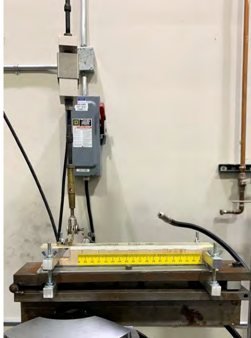
Figure 53. SCB test setup for delamination energy release rate determination, with Side A shown.
