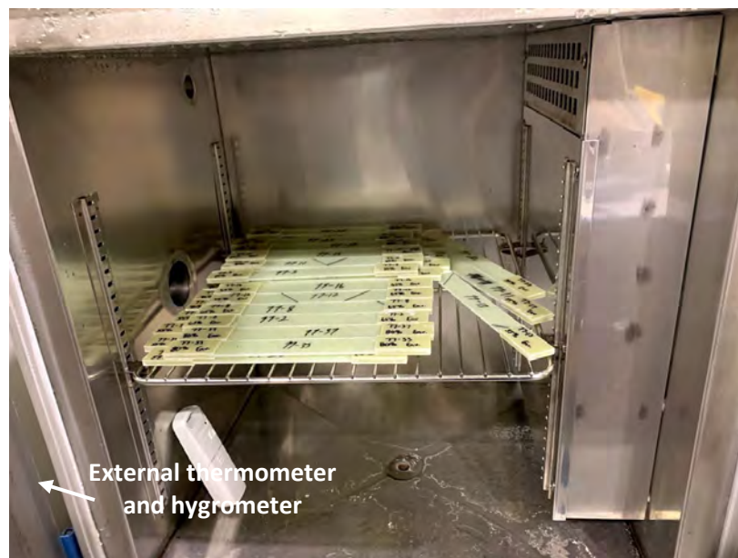
Figure 67. GF/Elium® coupons inside environmental chamber at 70°C and 90% RH.
