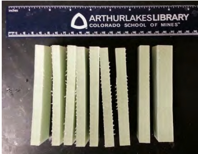
Figure 3. Strips of spar cap component (left) and subsequent ground composite material passed through a 3.5 standard mesh screen (foil pan) and a 7 standard mesh screen (round bucket).
