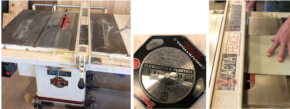
Figure 17. Jet tilting arbor table saw equipped with plexiglass blade used to rough cut samples.
