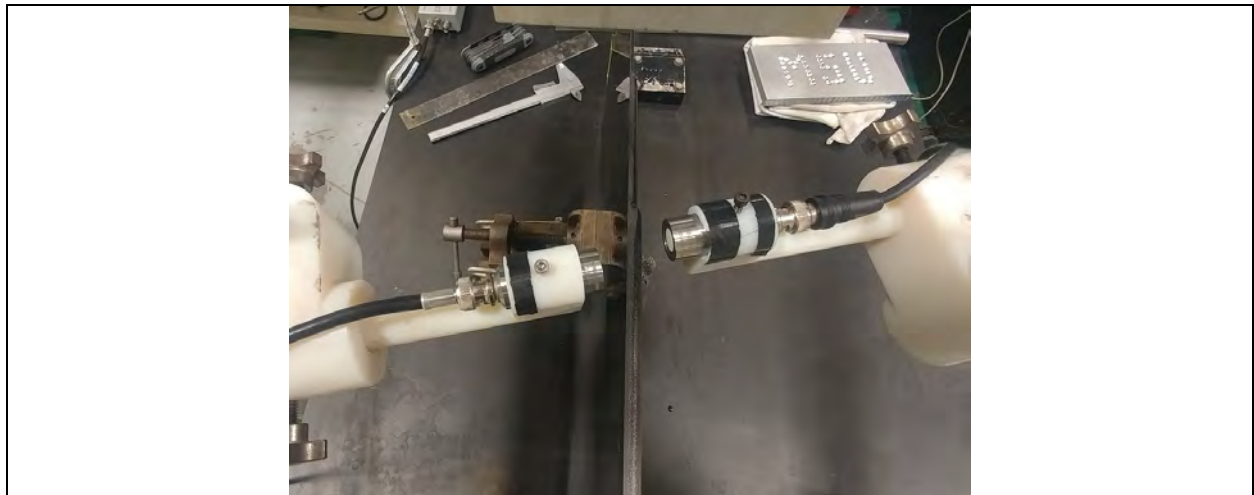
Figure 9. Scanning of calibration panel 1 in through-transmission mode at \theta_c = 14^\circ and 5 mm offset between the axes of air-coupled probes CF200.
