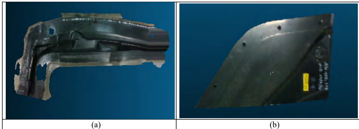
Figure 209. Stereo images of CFRP parts: (a) composite panel #3; (b) composite panel #4 (front splitter section) with embedded honeycomb structure.
