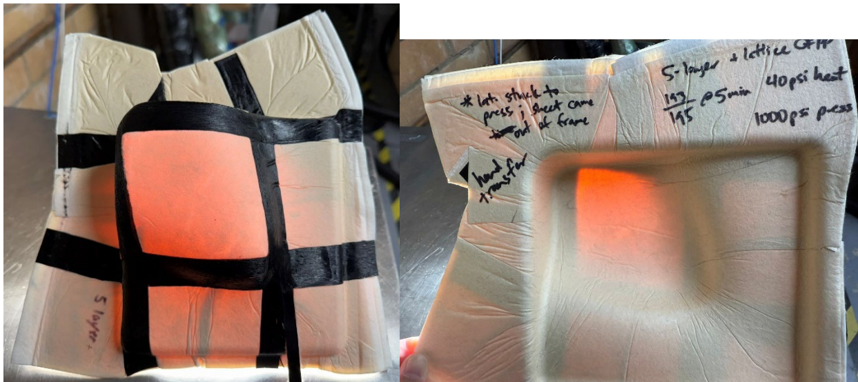
Figure 15: 5-layer cellulose nonwoven, 4 layers below lattice and 1 above, with GFPP lattice (25/25) backlight shows no tearing, as tapes are properly located on the stressed areas.
