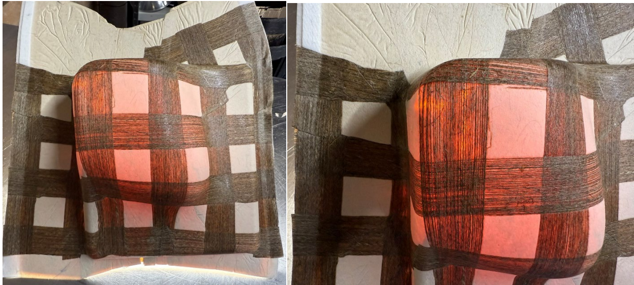
Figure 12: 5-layer cellulose nonwoven formed with NFPP lattice (50/50), backlight shows no tearing.
