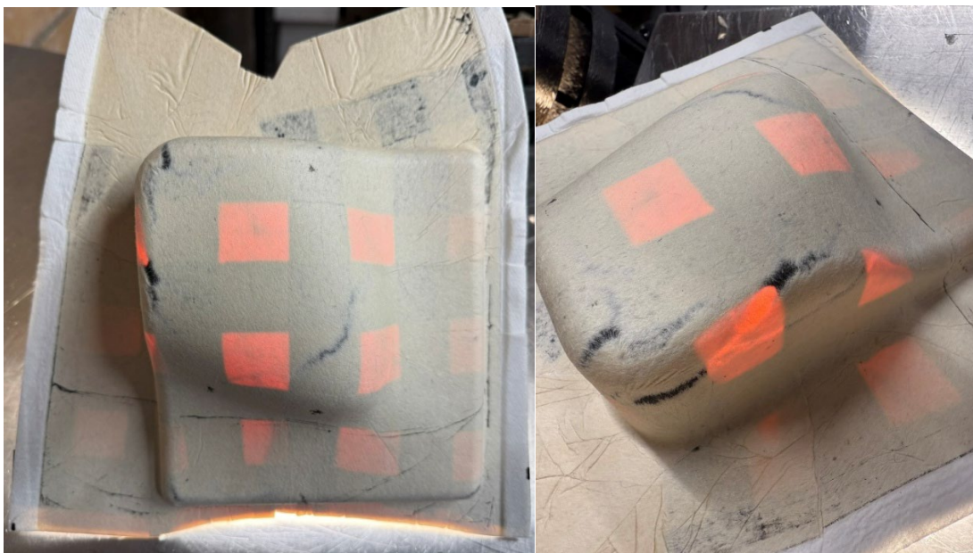
Figure 13: 5-layer cellulose nonwoven, 4 layers below lattice and 1 above, with GFPP lattice (50/50) backlight shows no tearing, but small surface tears are visible in the top cellulose layer.
