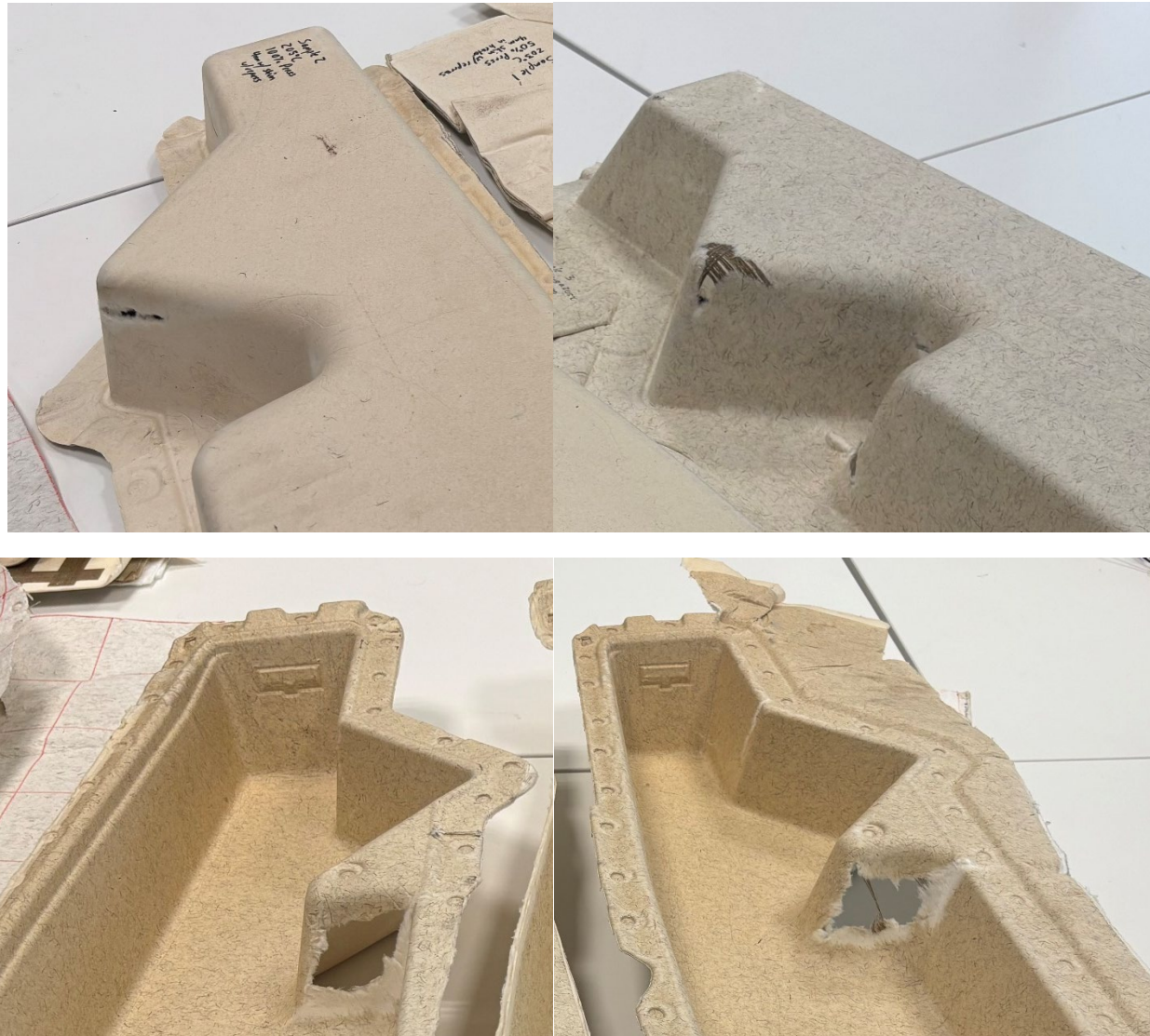
Figure 28: Comparison of control sample (Left) and NFPP lattice reinforced sample (Right) in higher complexity tool (deep draw, high complexity). NFPP lattice reduced through-tear of the sharp outer corner (Top Right vs. Top Left) but failed to prevent inner corner face tear (Bottom Right vs. Bottom Left).
