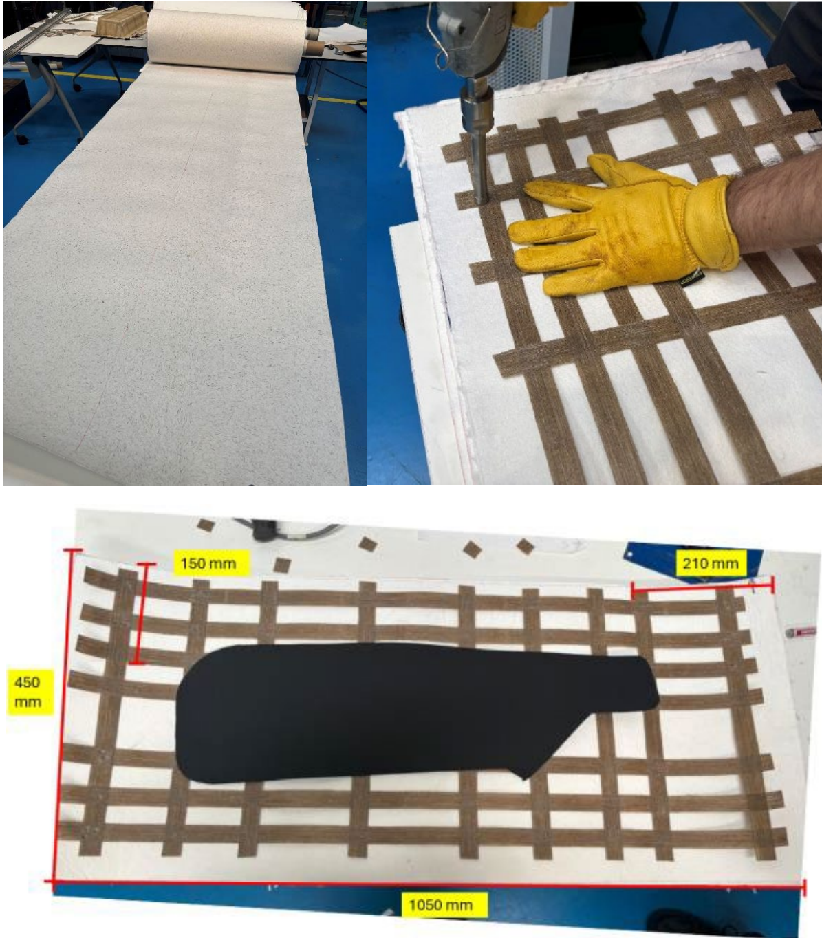
Figure 22: (Top Left) Marking of blanks from master rolls; (Top Right) Ultrasonic tack welding of lattice to blanks; (Bottom) Approximate alignment of tapes against top surface silhouette of part
