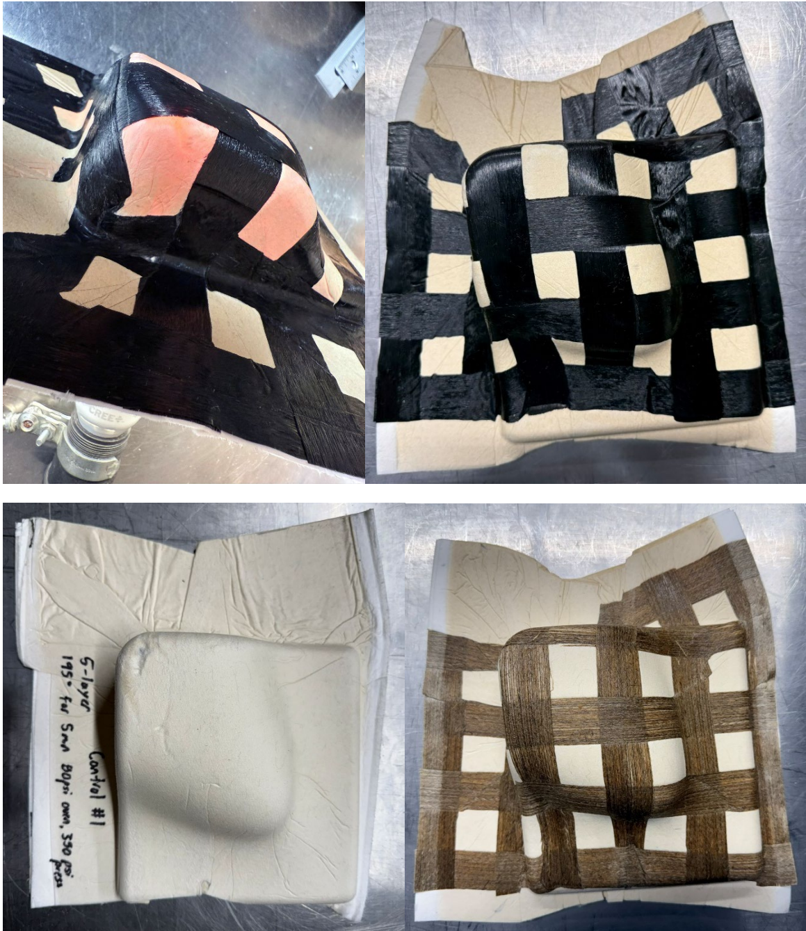
Figure 16: Comparison of overall wrinkling behavior. (Top Left) Close up of region with greatest wrinkling, note the discontinuity of the glass tape as it folds under the cellulose nowoven; (Top Right) GFPP lattice sample exhibits strong wrinkling at deep draw corner, single fold; (Bottom Left) Control sample exhibits strong, multifold wrinkling at deep draw corner, as well as minor wrinkles throughout the part; (Bottom Right) NFPP lattice exhibits strong, multifold wrinkling at deep draw corner.
