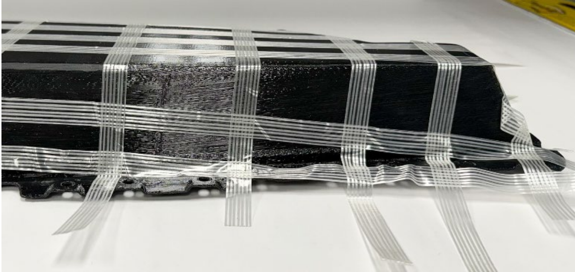
Figure 19: View of the least complex side of part, showing tape curvature on simple curves.
