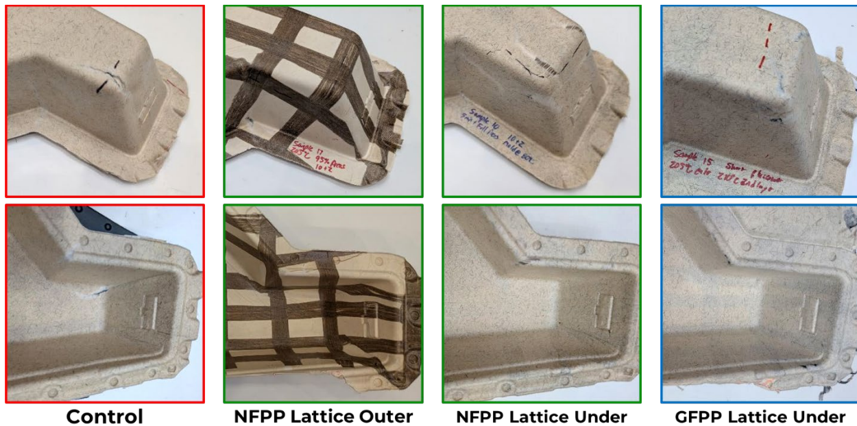
Figure 27: Close-up of complex corner features that exhibit major tearing in the control, but are fully controlled with the NFPP lattice on the outside, and only show surface layer tearing in the lattice under configurations.
