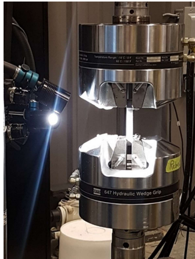
Figure 2.24: Tensile Test Setup.
