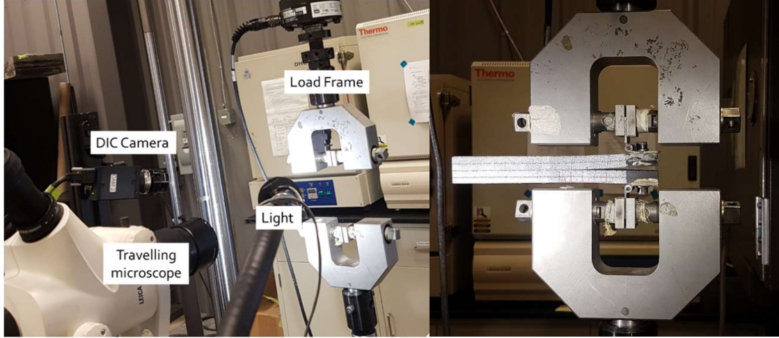
Figure 2.15: Setup used for testing DCB specimens in Universal Testing Machine.
