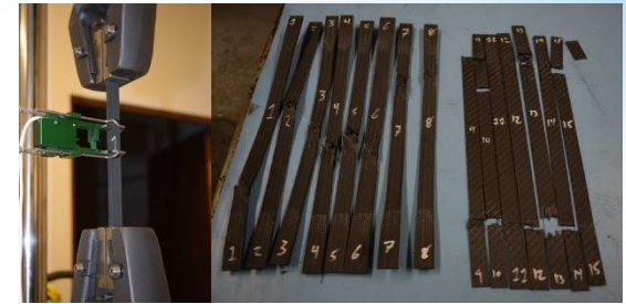
Test setup Specimens after testing: 8-ply shear, left vs. 4-ply tensile, right
