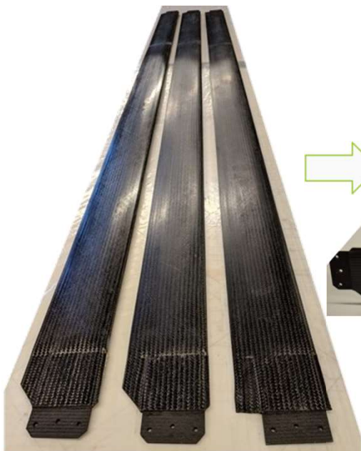
3 – 3.4m airfoils, tabs trimmed and ready to bend
