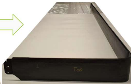
1 st bend completed at a specified distance from the end
